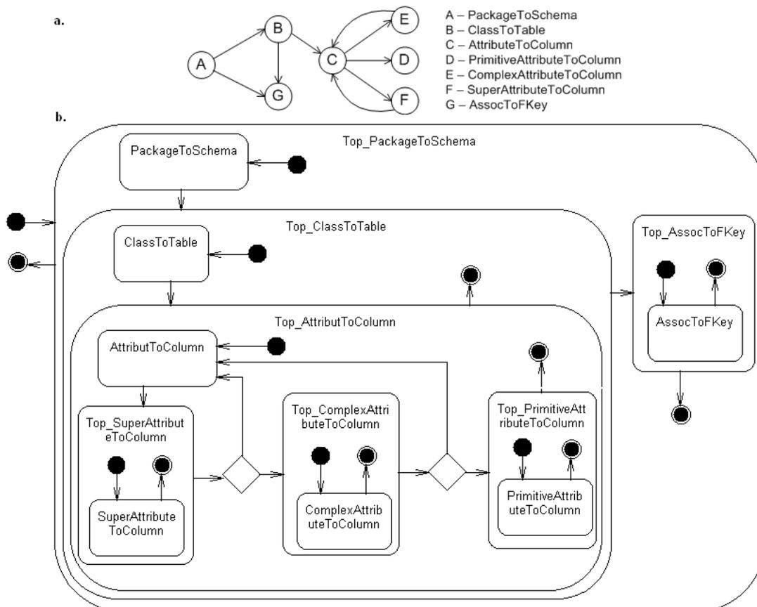
Figure 4: (a) Control Flow (CF) graph of the transformation *ClassToRDBMS* created by transformation *QVTConstructToVMTSConstruct*, (b) Generated VCFL model of the VMTS version of the transformation *ClassToRDBMS*
