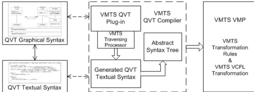
Figure 3: Overview of the QVT realization with VMTS
