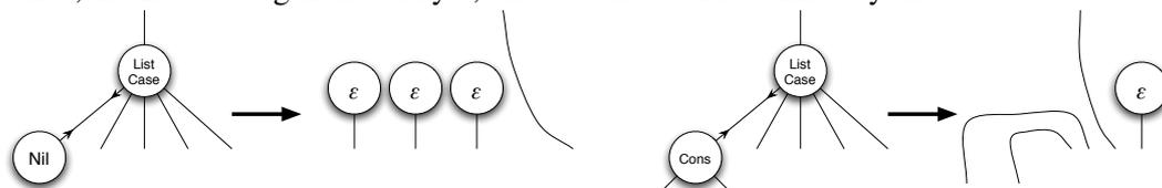
Here two different nets are connected to the ListCase agent. One is a net to be returned when the argument list is empty, and the other is a net with three ports, used to combine the head and
