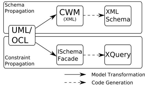
Figure 4: Mapping of UML/OCL-based domain models to XML
