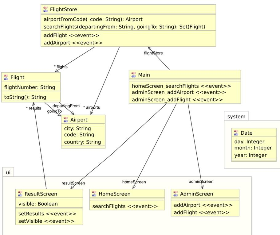
Figure 1: Class diagram of the FlightFinder application
