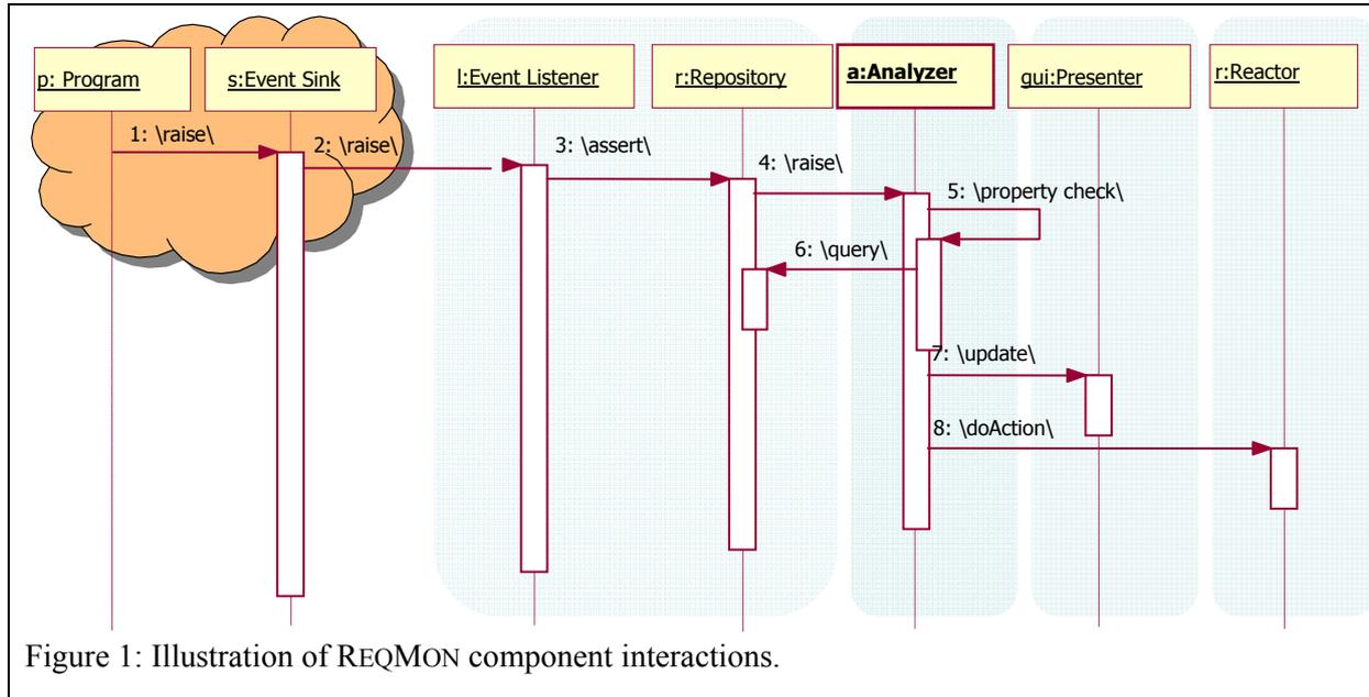
Figure 1: Illustration of REQMON component interactions.
