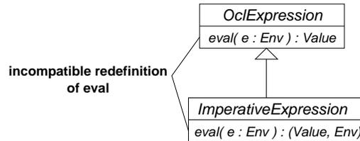
Figure 4: Problem illustrated using the OCL meta-model
