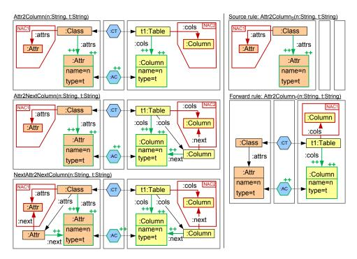
Figure 3: Rules for transforming attributes to columns and derived source and forward rule
