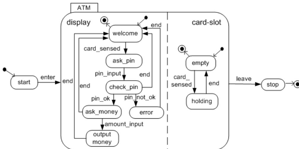
Figure 2: EMF instance graph: a statechart modelling an ATM
