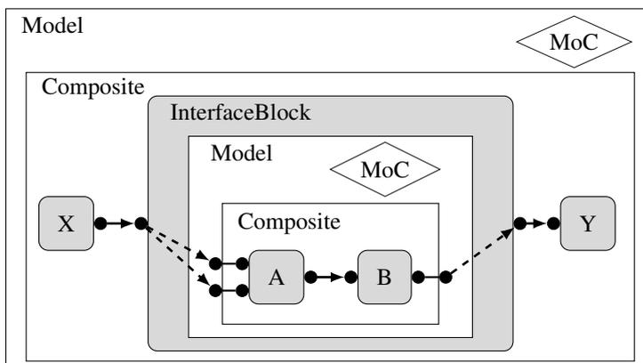
Figure 2: Model conforming to the meta-model of ModHel'X.
