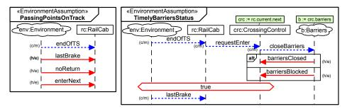
Figure 4: Assumption MSDs for the RailCab crossing example
