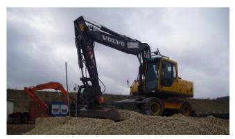
Figure 6: The autonomous mobile bucket excavator THOR
