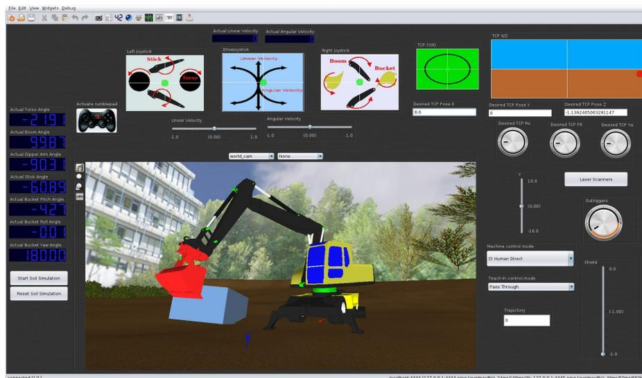
Figure 7: User interface created in FINGUI tool connected to simulated robot
