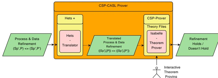
Figure 4: Diagram of the basic architecture of CSP-CASL-Prover.
