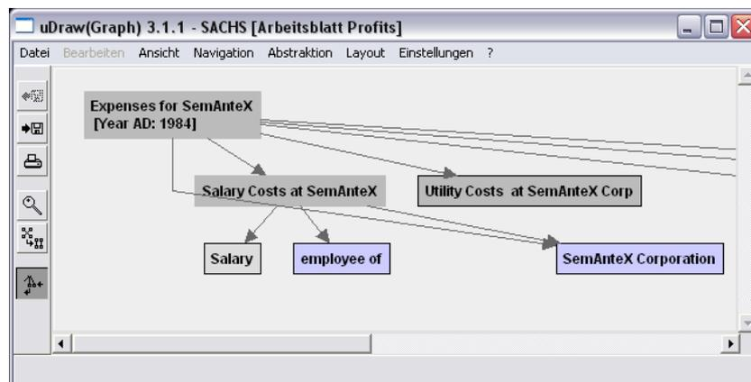
Figure 7: Dependency Graph for Cell [B15]
