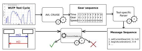
Figure 1: Possible Tool Chain for Validation of WLTP Gear Shift Sequences
