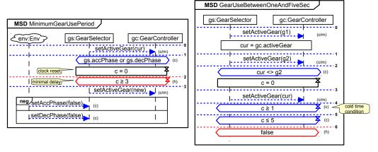
Figure 3: The MSDs MinimumGearUsePeriod and GearUseBetweenOneAndFiveSec (Req. (e))
