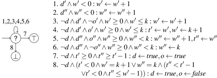
Figure 3: Observer for  $o \leftarrow \mathbf{X}^{kx}(o''\mathbf{U}^k o')$ . Initially  $t'' = 0, t' = -1, d = d_{\mathbf{X}} = false$  and  $w' = w'' = -k_{\mathbf{X}}$  (see text).
