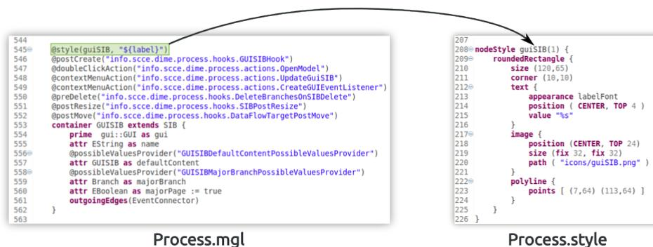
Figure 3: Excerpt of the MGL and MSL meta-model definition of the process type in DIME
