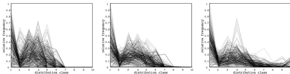
Figure 6: Distributions of the accelerator pedal positions for calm, normal and dynamic driving styles.
