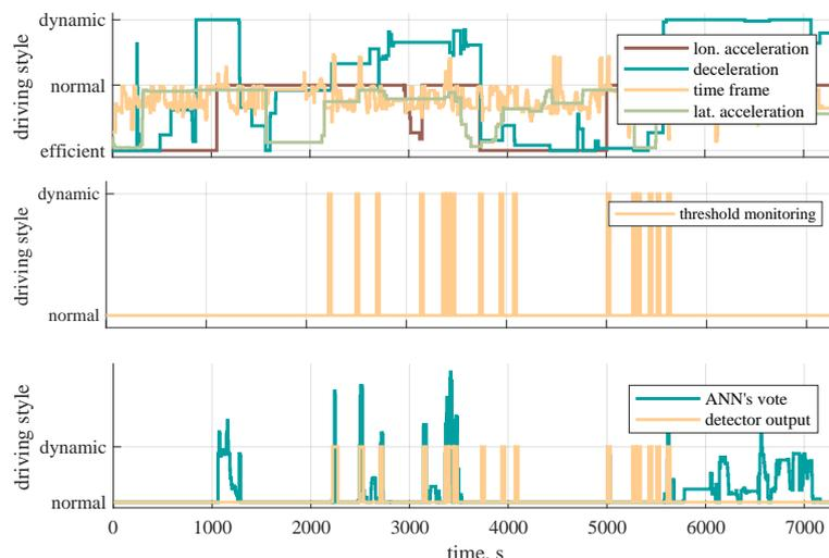
Figure 10: Output of the dynamic driving style detector during a test drive.
