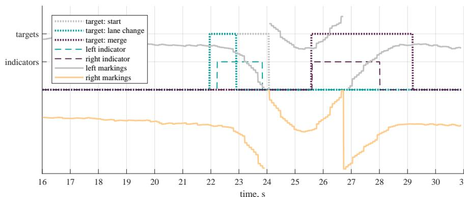
Figure 3: Overtaking maneuver represented by lane detection data and indicators showing the relative position of the data labels.
