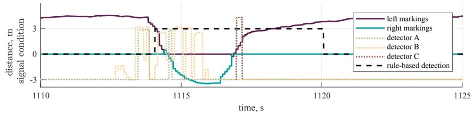
Figure 8: Output of the ANN-based and rule-based overtaking detectors.
