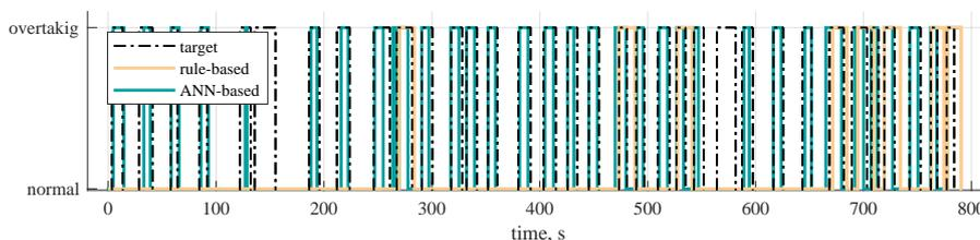
Figure 11: Direct comparison of the ANN- and rule-based overtake detectors.
