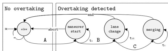
Figure 4: State machine representing overtaking maneuvers.
