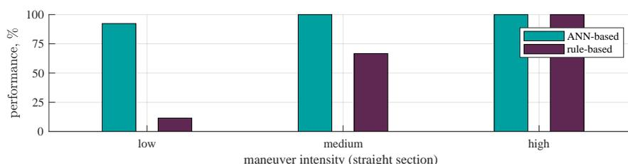
Figure 12: Results of ANN and rule-based detectors on straight roads.
