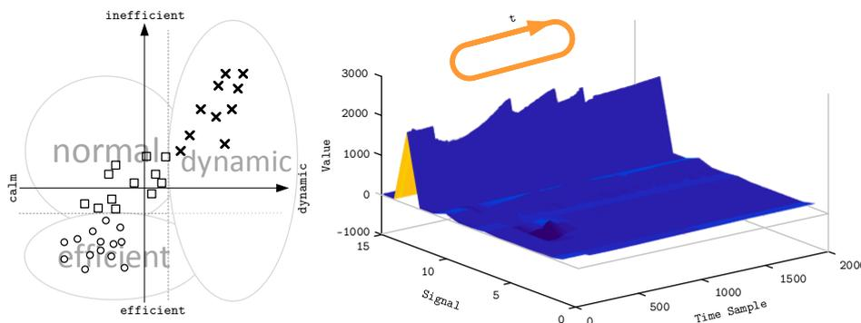
Figure 5: Left: Relative positions of driving styles {o, □, x} as a function of driving dynamics and energy efficiency. Right: Ring buffer containing 2000 samples of 15 different sensor signals.
