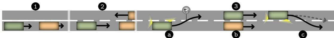
Figure 1: Phases of an overtaking maneuver.
