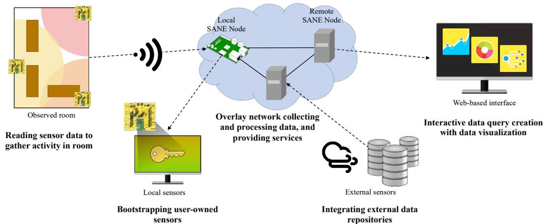
Figure 1: Demonstration setup showing locally deployed sensors, sensor bootstrapping, integration of external sensor data, and the interactive web interface to explore the SANE data space.
