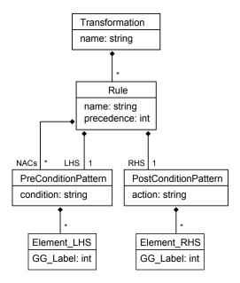
Figure 1: Structure of a transformation. Adapted from [KMS<sup>+</sup>10].
