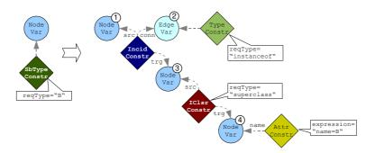
Figure 5: Definition of the SubTypeConstraint
