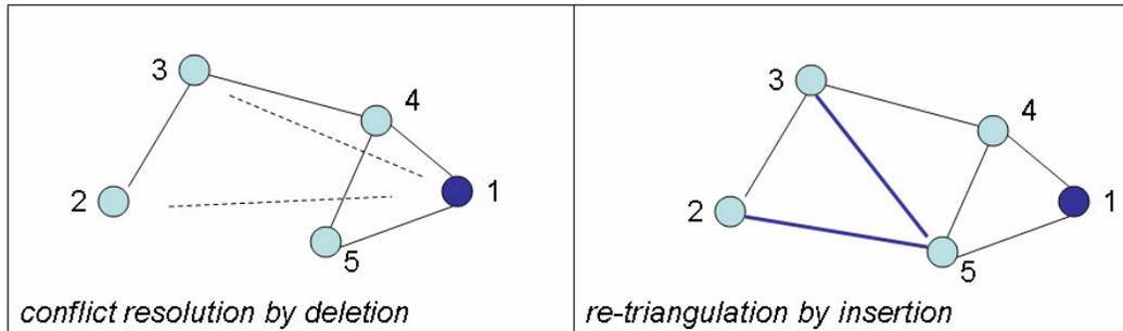
**Figure 9:** Continuation of the scenario of Figure 8. In a first step (left) the conflicting links are deleted (see dotted lines). Thereafter (right), new links must be established elsewhere to re-establish the desired triangulation property (see thick blue lines).
