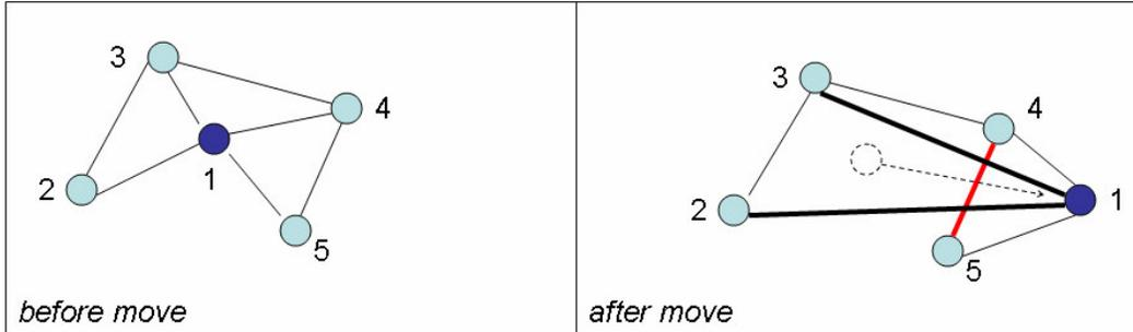
**Figure 8:** Scenario in which the triangulation property is violated after a far-reaching move of unit 1 (see red line). The edges between units 1 and 2, respectively units 1 and 3, are now crossing the edge between units 4 and 5, such that this sub-graph is not planar any more.
