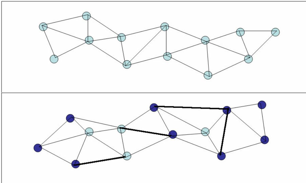
**Figure 1:** Triangulated network before (top) and after (bottom) the movement of some nodes. Dark shaded nodes have changed their positions, and some communication links have also been reconfigured in their topological positions, which is depicted by thicker lines.
